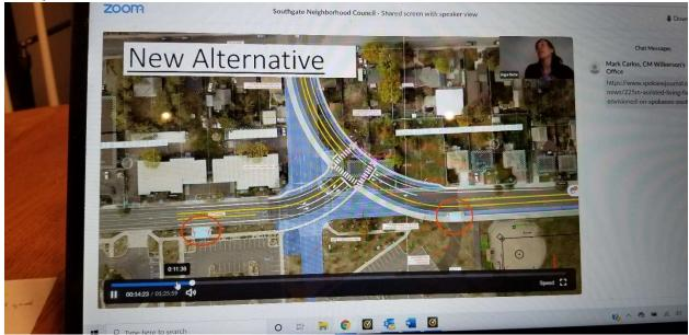
❖ New alternative B: Roundabout at 37<sup>th</sup> and Ray but moves the intersection to the East. The Ferris exit is not included in the roundabout. Analysis of this alternative will also be done.
